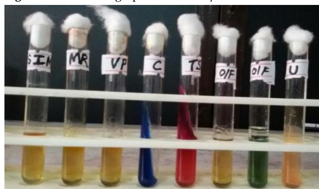
Figure 2: Biochemical test of P. aeruginosa (From left to right: SIM sulphite “- ve”; Indole “- ve”; Motile; MR “- ve”; VP “- ve”; Citrate “+ ve”; TSI Acid/no change; O/F “Oxidative”; Urease “- ve”).
