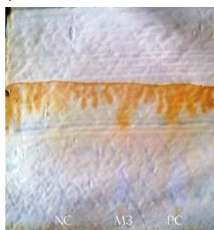
Figure 2: TLC of extracted metabolite from M 3 isolate Note: NC: Negative Control; M 3 : Secondary metabolite from M 3 isolates; PC: Positive Control (gentamicin)
